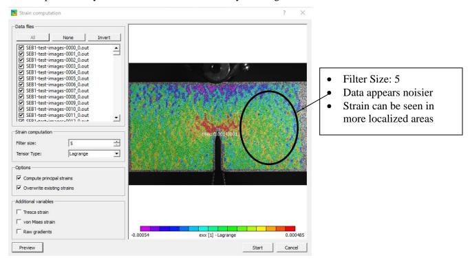
When using a larger strain filter, the strains will be cleaner, however we lose some resolution for local strains. The same data as above list shown below with a larger filter size of 35.
