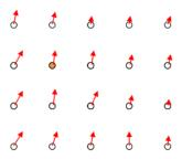
The separation between these points (in pixels) is dictated by the step size. The separation between the points in physical space will vary depending on magnification and the shape of the specimen. With this grid as the input, we consider each point separately, and create a local mesh of triangles; here, we consider the highlighted point from above:
